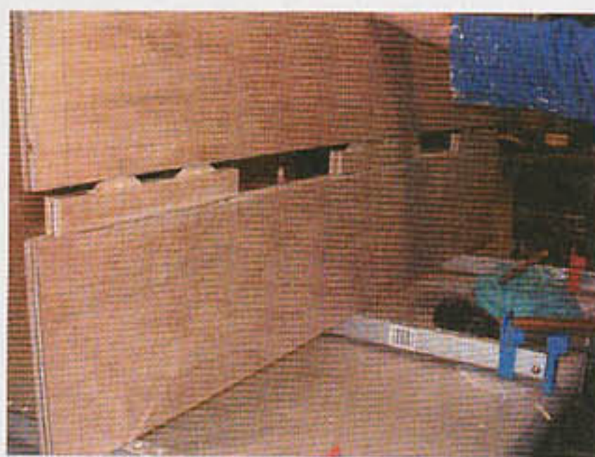
Joining the table top sections with biscuits and adhesive
