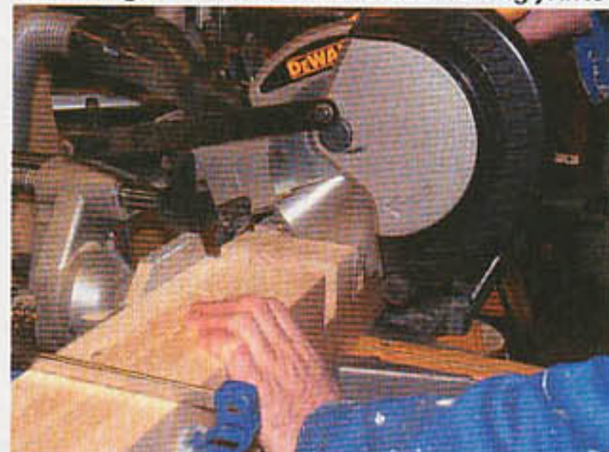
Trenching out the stretcher cross-halving joints
