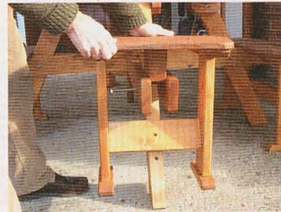
Make sure that the bolt is fed through the first stretcher before lowering the small seat into position
